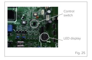
Press the control switch to open the unit's information menu. The first code "00" is shown on the LED display. Press the switch again to display code "01". After 1.5 sec the code displayed alternates with its respective value. When the switch is pressed again, the next code is displayed.
