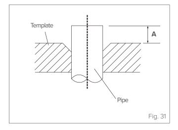
**8** Remove the countersunk screw and template, then check that the end of the pipe is countersunk evenly and not cracked.
