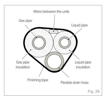
Gas pipe insulation: minimum thickness 13mm Liquid pipe insulation: minimum thickness 10mm
