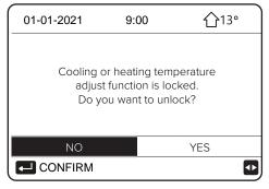
The cooling/heating mode cannot be switched on or off when COOL/HEAT ON/OFF is locked.
