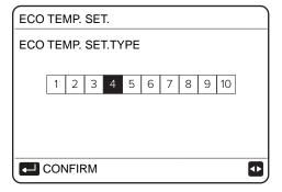
Press ON/OFF to select on/off, press Up, Down to scroll.
