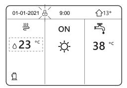
If the interface is unlocked, long press the UNLOCK button  $(\stackrel{\Omega}{\cup})$  to lock the interface.
