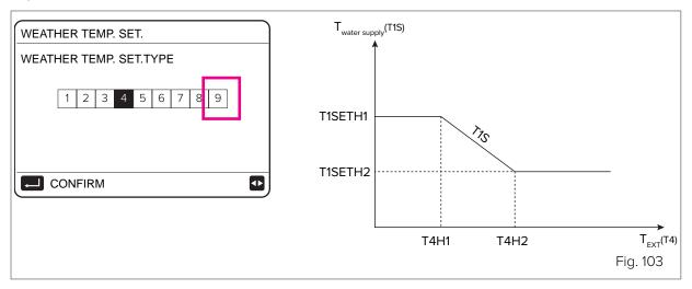
• 8 default curves for Cooling mode on systems with radiant distribution.
