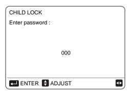
Press Down, Up to scroll and press ON/OFF to lock or unlock one or more operation modes.
