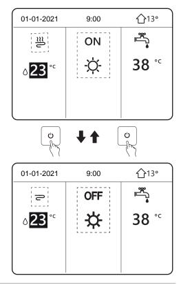
If DHW MODE SETTING is set to NO, the following pages will be displayed without the DHW function.
