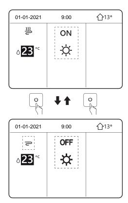
The room thermostat can be used to switch the unit on or off for heating or cooling the room.
