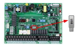
With the unit powered and switched **Off** plug the flash drive into the USB port on the indoor unit board.
