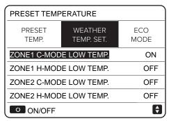
If WEATHER TEMP. SET. is on, the temperature cannot be adjusted.
