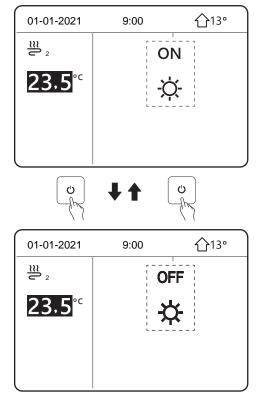
On the interface it is possible to switch on or off the unit for domestic hot water production.
