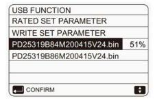
Select the file for the indoor unit. When the procedure has finished, the word "**SUCCESS**" is displayed.
