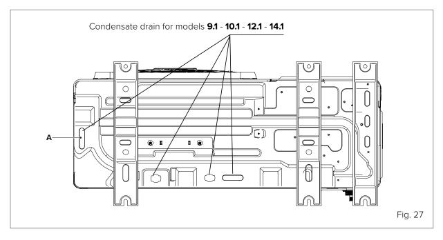
The drain hole (A) is covered by a rubber plug. If the smaller drain hole cannot fulfil the drainage requirements, the larger drain hole can be used at the same time.
