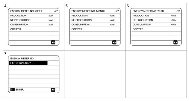
Note: "Hour" display shows the real-time calculated values. Instead for the other period the value are the result of the integration of the corresponding power values.
