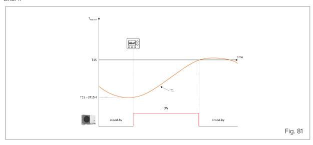
This value is strongly related to the minimum permissible water content of the circuit. A narrower control band can be accepted with a high water volume.
