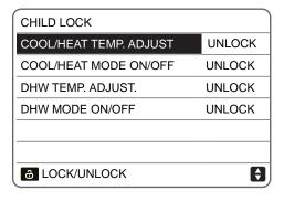
If you want to adjust the cooling/heating temperature when it is locked, the following page appears.
