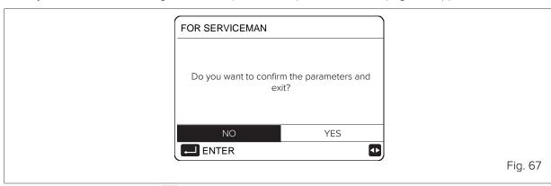
Select "YES" and confirm with to save the settings and exit. After exiting, the unit will shut down.
