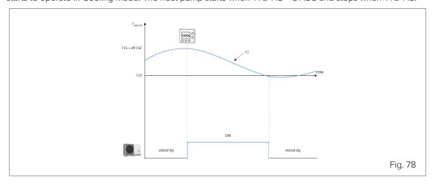
This value is strongly related to the minimum permissible water content of the circuit. A narrower control band can be accepted with a high water volume.
