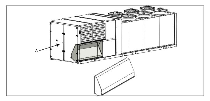
Open panel A, inside there is the hood and the fixing screws.
