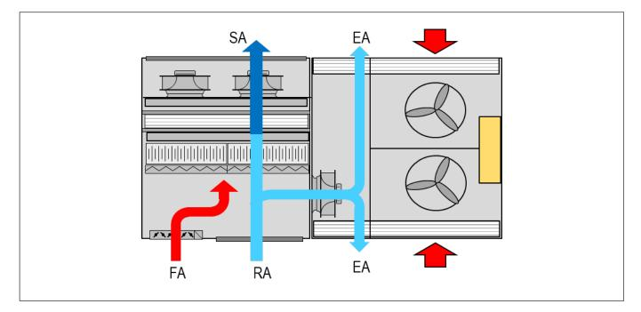
Double fan section with fresh air and REVO thermodynamic recovery
