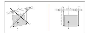
Align the barycenter to the lifting point
