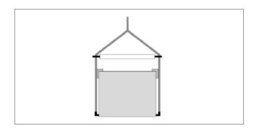
Lifting with spacer bar
