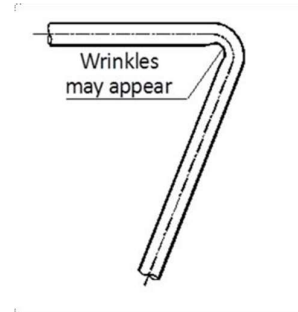
Figure 3-4.3: Pipe bending in excess of 90^\circ
