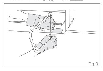
**3** Remove any burrs along the cut section using a half round file.
