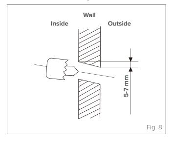
**3** Insert the protective sleeve into the wall, which will protect the edges of the hole and improve the seal after installation.
