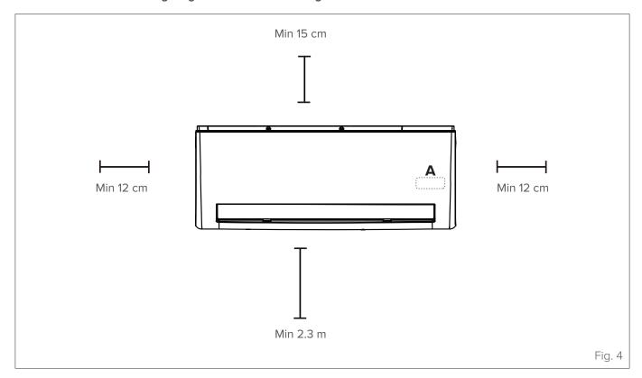
A Position of the display EZCool and remote control signal receiver.
