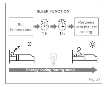
Cooling mode (+1°C) per hour for the first 2 hours Heating mode (-1°C) per hour for the first 2 hours
